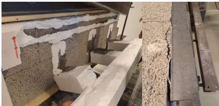
Fig. 9. FIBO wall construction after tests
